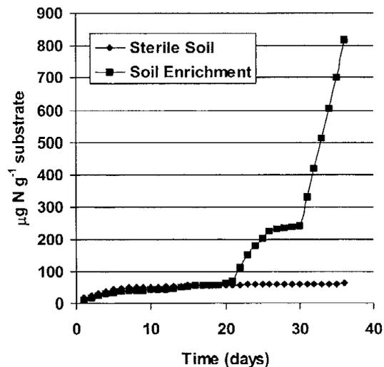
Figure 6. Nitrite-oxidation based on cumulative  $\text{NO}_3^-$ -N leached from columns containing zeoponic substrate inoculated with soil enriched for nitrifying bacteria, and an uninoculated control.
