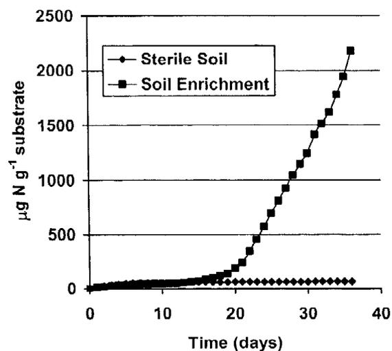
Figure 5. Gross  $\text{NH}_4^+$  oxidation based on cumulative  $\text{NO}_2^-$ -N and  $\text{NO}_3^-$ -N leached from columns containing zeoponic substrate inoculated with soil enriched for nitrifying bacteria, and an uninoculated control.
