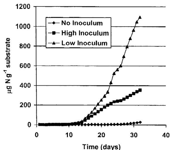
Figure 3. Cumulative  $\text{N}_2\text{O}_2^-$  -N leached from columns containing zeoionic substrates receiving two rates of inoculation, and an uninoculated control.
