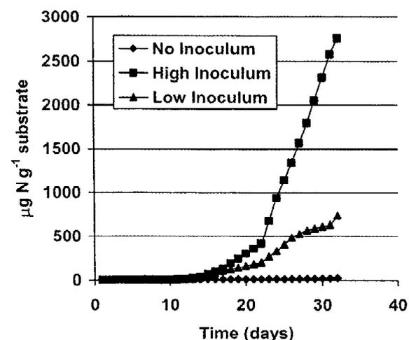
Figure 2. Nitrite-oxidation based on cumulative  $\text{NO}_3^-$  -N leached from columns containing zeoionic substrate receiving two rates of inoculation, and an uninoculated control.
